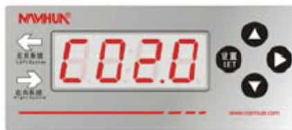
Fig.2 Alarm point setting
