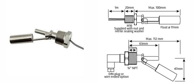
The 80 Series is a small horizontally mounted liquid level sensor designed for high temperature/high pressure operation and sensing chemically aggressive liquids. The design provides a highly cost effective solution where high reliability in a demanding environment is called for.
