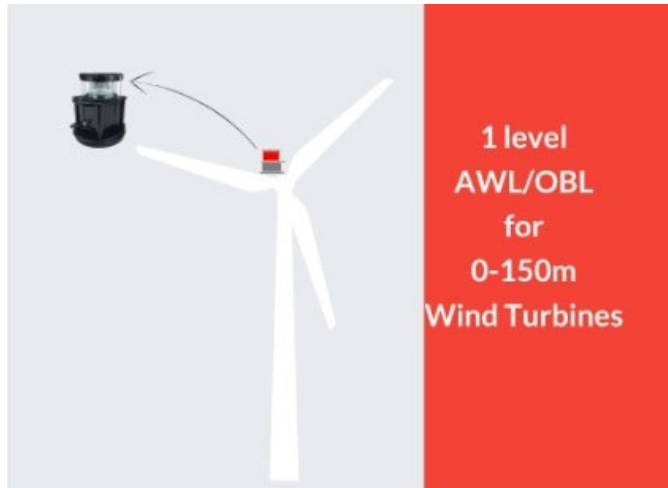
WT150E-1F864 Medium Intensity Aviation Obstruction Lighting System for wind turbines
