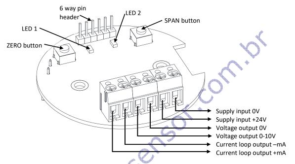
The sensor outputs the liquid level as a varying voltage or varying current. Connection can be made to voltage, current or both voltage and current outputs.
